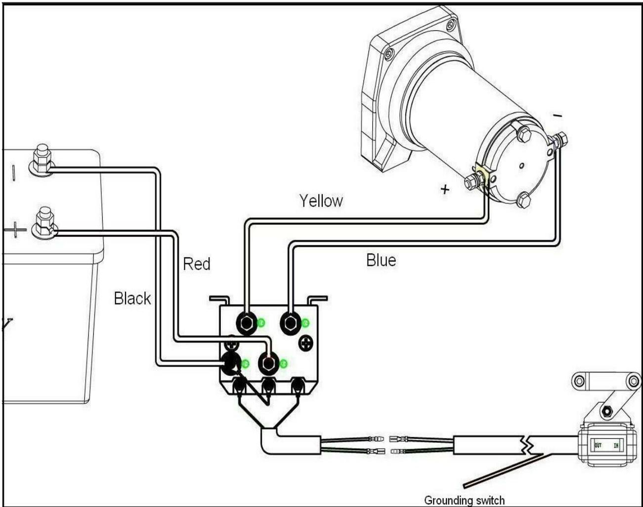
Figure 7 Wiring instalation diagtam
