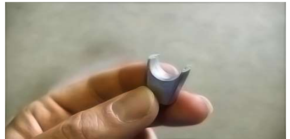
**OEM sample of failed dump box shock eyelet**
